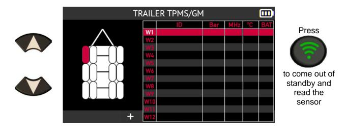
The tool brings the trailer's first sensor out of standby and reads the information it contains.
