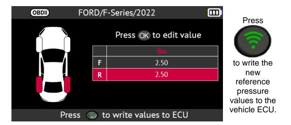
The new reference pressure values are recorded in the vehicle's ECU. The VERIFY OK message confirms the data have been saved.
