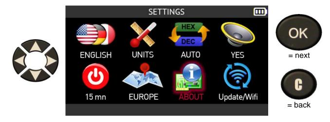
The **About** screen is displayed. This displays the tool's serial number, the firmware and database version numbers and the validity of the software licence.
