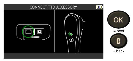
Check that the **Tire Tread Depth gauge** indicator light is green.
