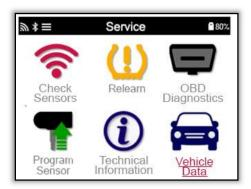
The menu gives direct access to specific screens that display the Vehicle data. This option is helpful if the user wants to have a second look at the Sensor Data, OBD Data or wants to print the data from the last processed vehicle via the Bluetooth printer.
