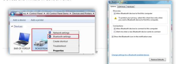
Right click on the Bluetooth dongle icon and click on Bluetooth settings. Tick the boxes as seen on the Options tab above. Press OK when finished. Start the TPMS Desktop application and go to Settings. Open the Bluetooth section: the PC/Laptop should be **connectable** and **discoverable** for the TECH600.
