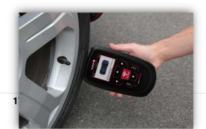
(Note: with Ford Banded sensors the tool should be held 180°/opposite from the stem's position)
