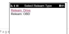
To find out which relearn type is available for a vehicle, just turn on the tool and select Relearn. Or refer to the current coverage list at <a href="https://www.bartecautoid.com">www.bartecautoid.com</a> > Downloads.
