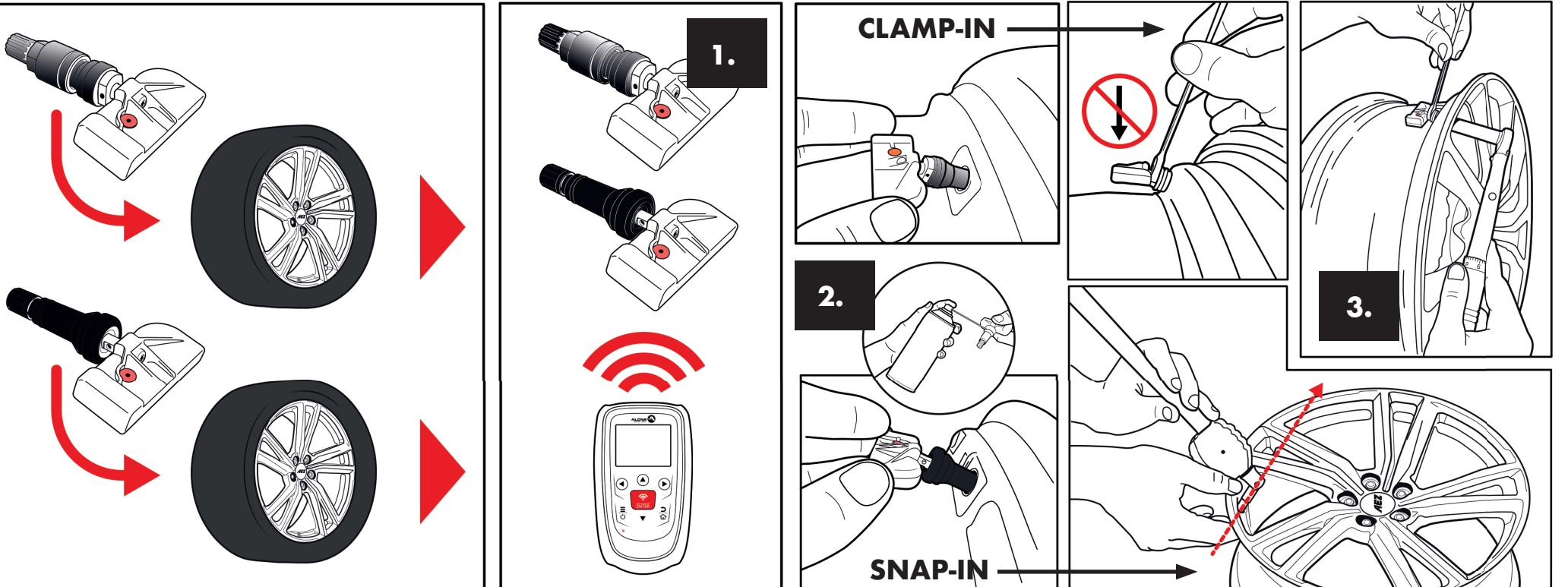
**EN:** ALCAR recommends exchanging all relevant components of TPMS valves when changing tyres to ensure the functionality of the TPMS system and the safety of all passengers. To prevent damage during replacing also note the required tightening torques of the individual components.
